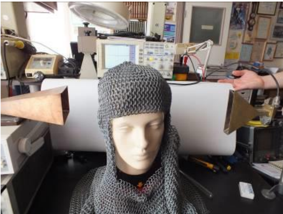
Figure 3: "Free-space" measurement technique
