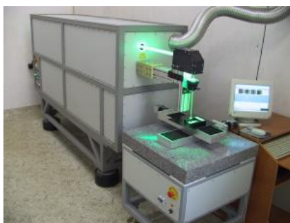
Figure 2: a) A laser system with CuBr used in the 'Pulslight' company [154] b) Schematic diagram of a laser tube: 1-tanks with copper bromide, 2-thermal insulation on active volume, 3-copper electrodes, 4- inner diaphragms, 5 - output windows [12,13].
