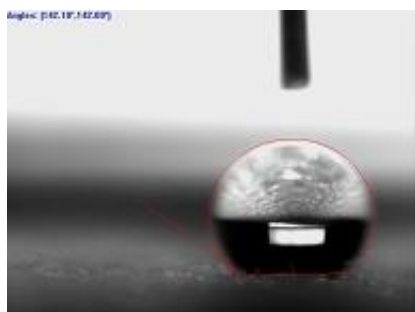
Figure 2 – Contact angle measurement on cotton fabrics
