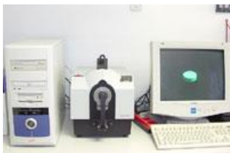
Figure 3: Spectrophotometer „Datacolor SF 300” [20]
