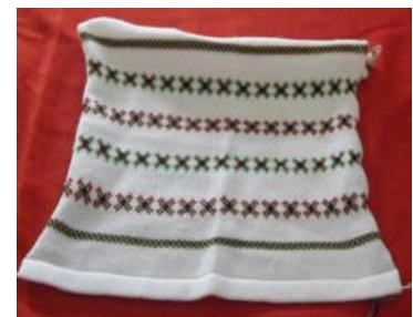
Figure 19: Geometric folkloric motif transposed in a knitted structure with a full jacquard design on one frame
