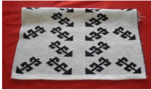
Figure 15: Partial jacquard structure in two colours with skeuomorphic folkloric motif – plough stilt
