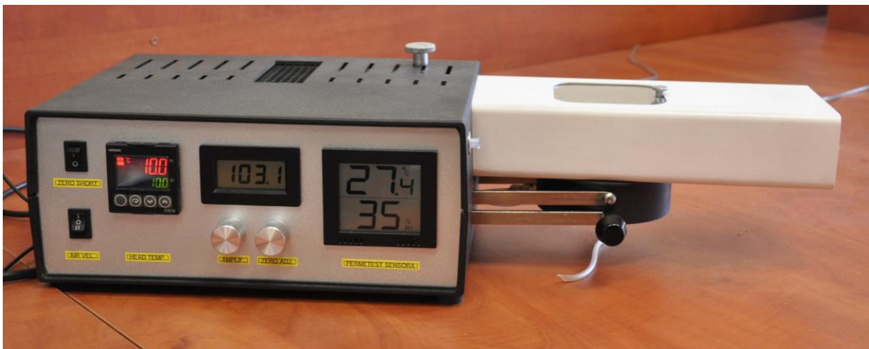
Figure 5: The PERMETEST Skin model, a non-destructive tester of water vapour permeability of fabrics
