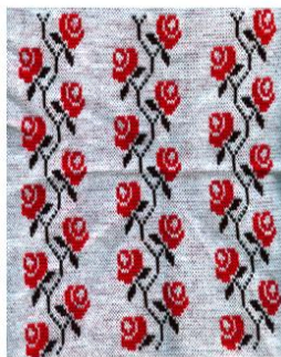
Figure 5: Folkloric floral model transposed in knitted structure as a full jacquard design in 3 colours
