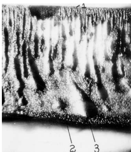
Figure 3: Micrograph SEM (30x) of the PU membranes obtained by phase inversion in water at 25°C [2, 3]. 1 - contact surface with nonsolvent (water); 2 - substrate surface; 3 - micropors.
