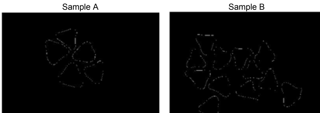
Figure 5. Binary image segmentation with Canny algorithm
