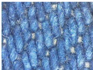
Front side of the denim fabric (weave twill 3/1)
