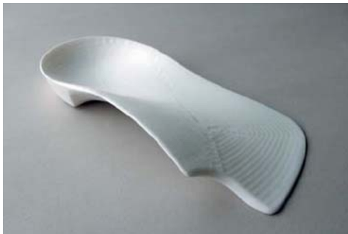
Figure 7: 3D orthoses model built on a CNC milling machine
