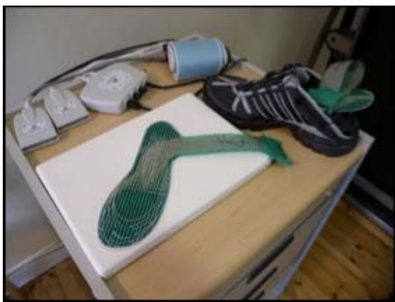
Figure 2: In-shoe pressure data collecting system
