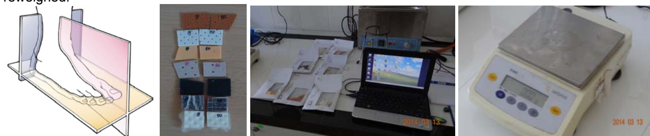
Figure 3. Weighing samples, symmetrically cut from sagittal plane (along the leg) [10]
