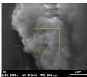
Figure 16: Map of the specific elements distribution for PU+ZSM-5+ kevlar composite obtained using the inversions method in dry phase
