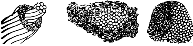
Figure 6: Schematic presentation of core yarns
