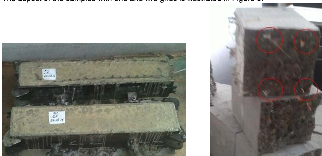
Figure 3: Samples of concrete reinforced with yarn grids Figure 4: Aspects of the samples after testing
