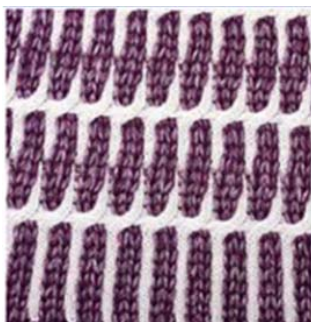
Figure 3: Effect of dynamic stitch length/cast-off
