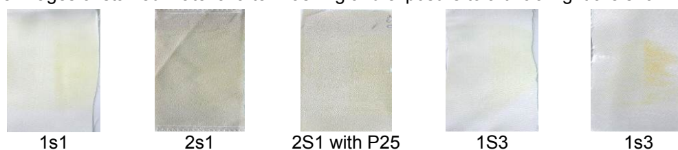
Figure 11: The images of stained material after washing and exposure to artificial light. The results show that samples Satin and Crepe sputtering and electro spray with TiO 2 and TiO 2 /Ag 1% were partially cleaned and samples Crepe sputtering with TiO 2 P25 Degussa cleaned well.
