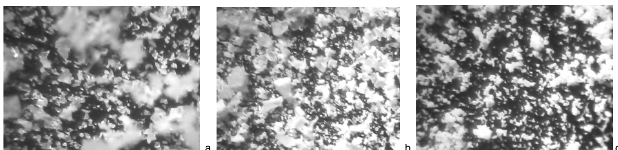
Figure 2. Microscopic images of dry hydrolysates: a) normal hydrolysis; b) electrolytic hydrolysis at 6 V; c) electrolytic hydrolysis at 6 V.
