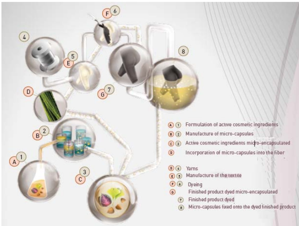
Figure 3: Manufacturing process of a cosmetic textile
