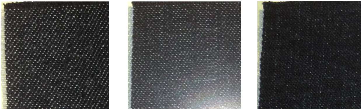
Figure 1: Images of the denim fabric samples before finishing, after finishing and after washing
