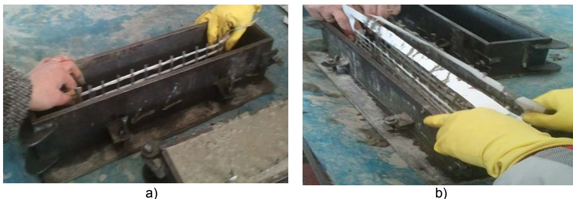
Figure 2: Positioning the grids in the samples
