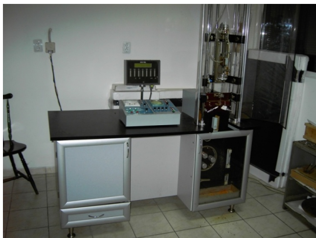
Figure 3: Production equipment for the microyarns (INCDIE ICPE-CA)
