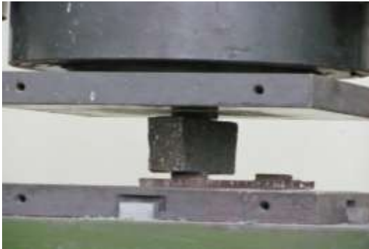
Figure 9: Polymeric concrete tested for split tensile strength
