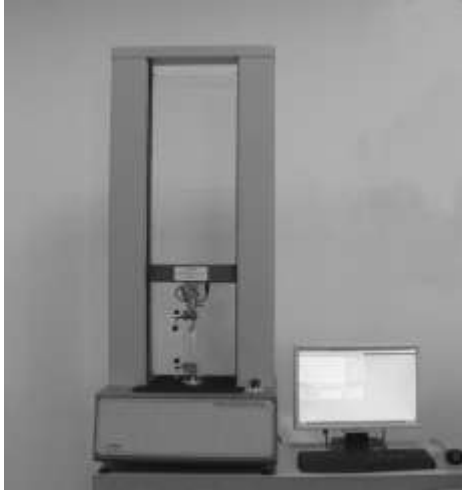
Figure 1: The tensile testing machine SATRA with 466F attachment
