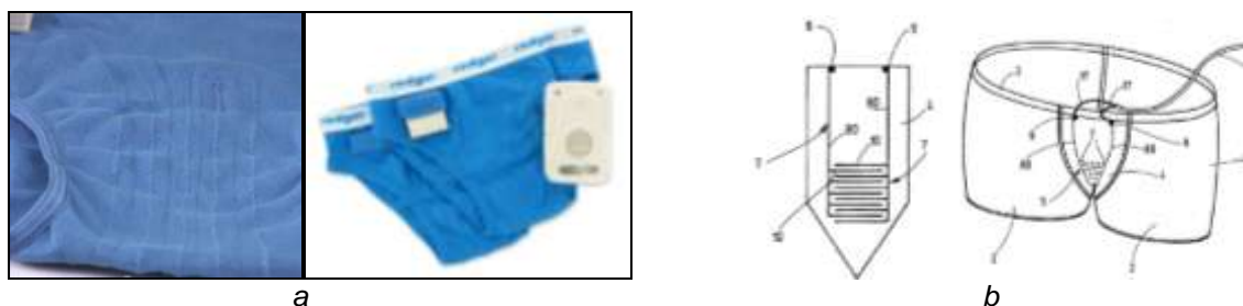
Figure 4: Title of figure: a - Rodger wireless alarm; b - pants with conductive threads as the sensor
