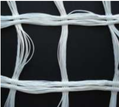
Figure 4: Knitted geogrid variant 2 – fabric aspect (before and after impregnation)
