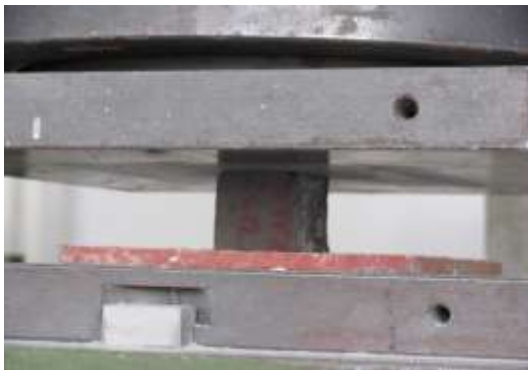
Figure 5 Fibre reinforced concrete tested to axial compression
