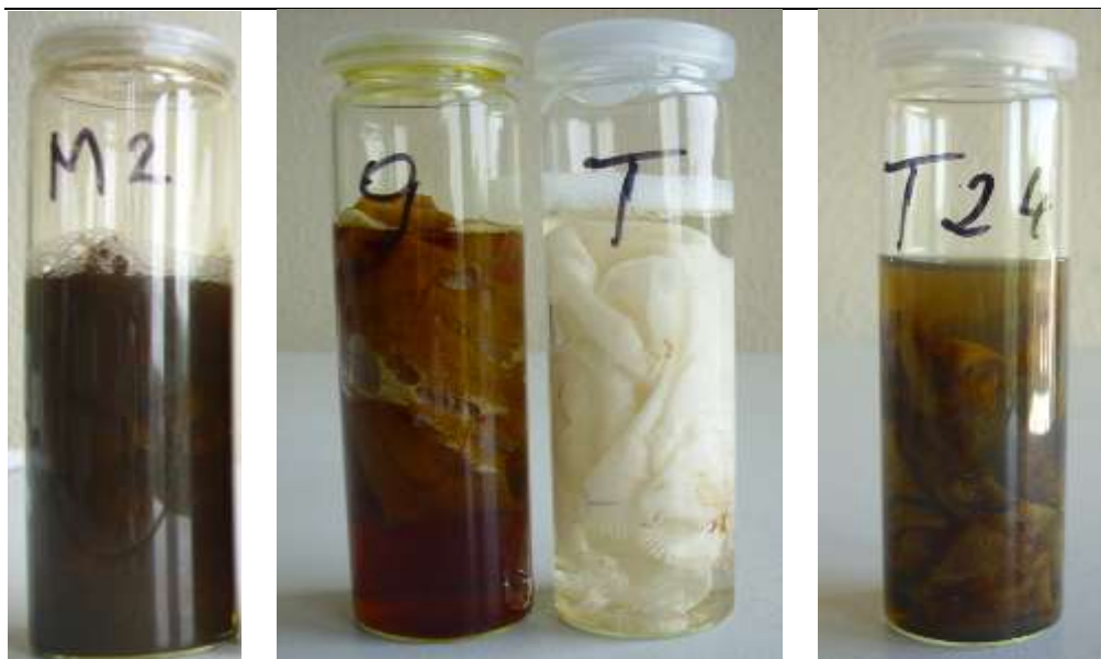
Figure 1: Appearance of fabrics and reducing silver bath for the ungrafted fabric with MCT- \beta -CD (Sample M2), fabric grafted with MCT- \beta -CD (Sample 9), fabric grafted with triazine (Sample T) and fabric treated with triazine after 24 hours at 50 °C (Sample T24)
