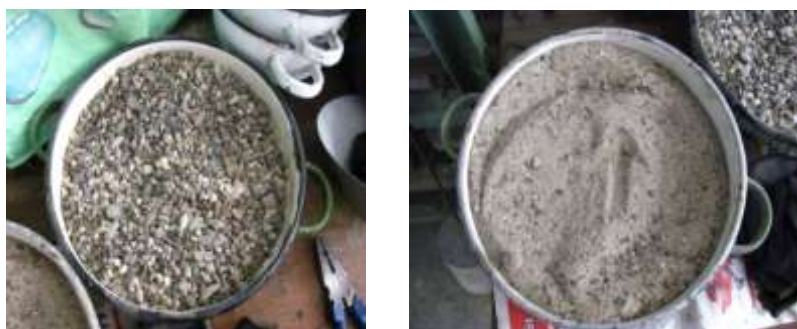
Figure 1: Crushed aggregates: 0-4 mm –sort I and 4-8mm – sort II
