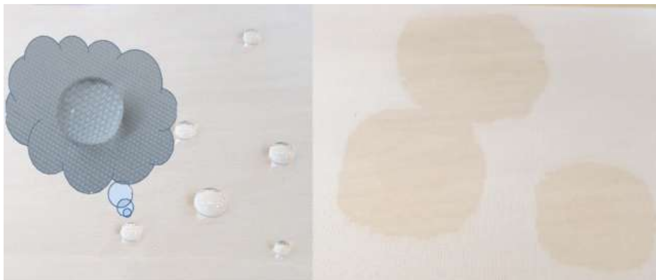
Figure 5: Treated and untreated PES fabric with Ruco-Dry Eco solution.
