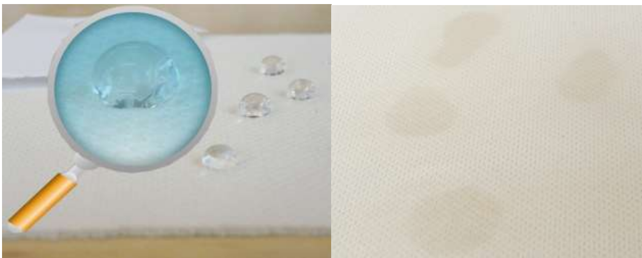
Figure 6: Treated and untreated fabric spacer 100 % PES with Ruco-Dry Eco.
