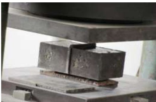
Figure 7 Fibre reinforced concrete tested for flexural strength (fti)
