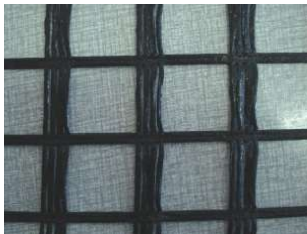
Figure 2: Knitted geogrid variant 1 – fabric aspect (before and after impregnation)
