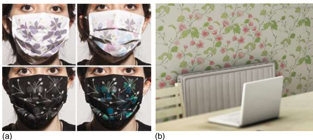
Figure 1: Thermochromic textiles that change colour with temperature (a) fashionable flu-masks and (b) blossoming wallpaper
