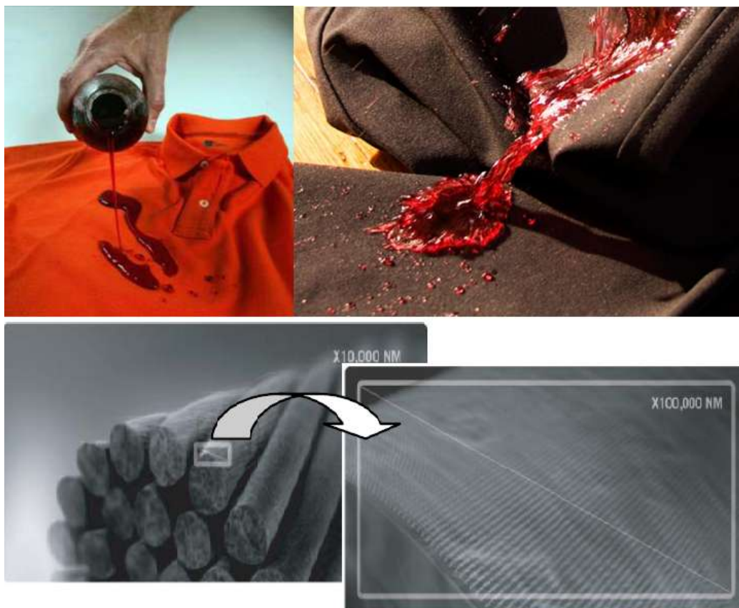
Figure 1: Nano-Tex ® Resist Spill fabrics with superhydrophobic properties and high magnification images of the fibers surfaces.
