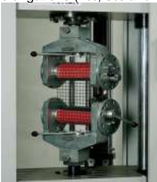
Figure 5: Tensile testing of the geogrids - Tinius Ohlsen 25kN machine
