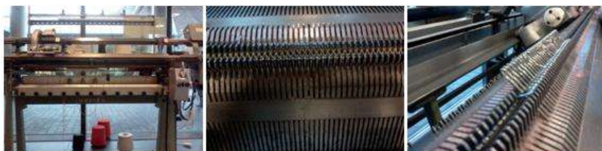
Figure 1: Production process for the single jersey knitted samples, using a Dubied flatbed knitting machine
