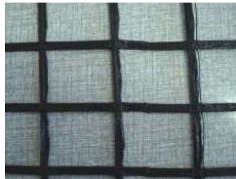
Figure 4: Knitted geogrid variant 2 – fabric aspect (before and after impregnation)
