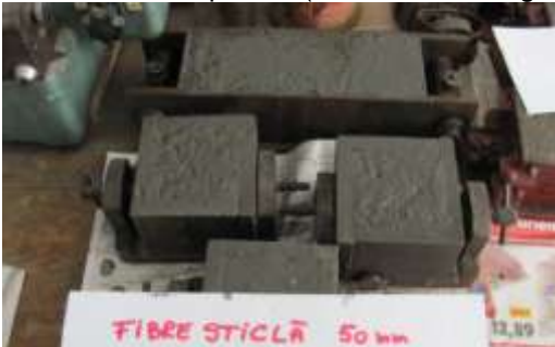
Figure 4: Samples of fibre reinforced concrete - glass fibres, 50 mm
