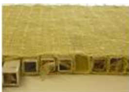
Figure 2: U shaped sandwich knitted fabric
