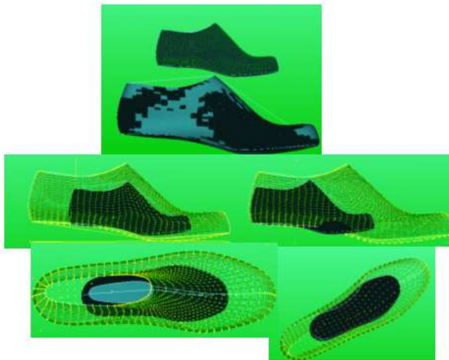
Figure 6 : The result for compare LAST1 with LAST2 beyond modification the parameters of the last 1 in parameters of the last2
