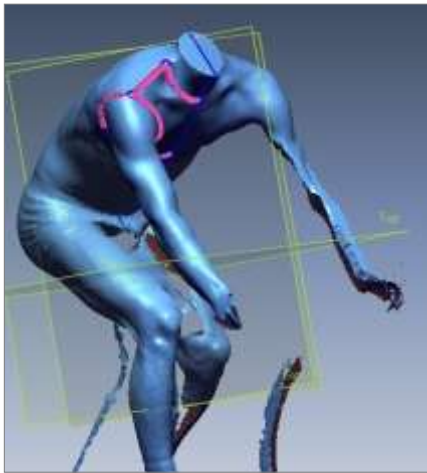
Figure 7: 3D morphology (bike position) obtained by scanner and corrected by CAD software
