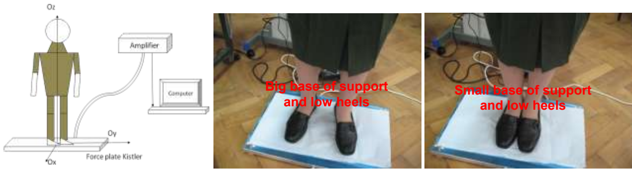
Figure 2: Experimental setup used to record bipodal stability and recording example
