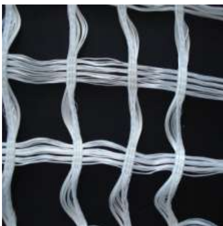
Figure 2: Knitted geogrid variant 1 – fabric aspect (before and after impregnation)
