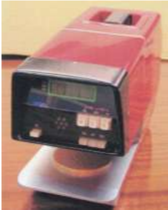
Figure 9: Computer-controlled instrument ALAMBETA for the fast measurement of thermal insulation and thermal-contact properties of any compressible materials, especially plain textile fabrics. The instrument measures the sample thickness also. Results are statistically treated.
