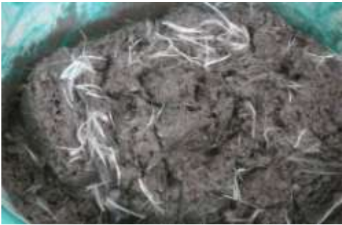
Figure 3: Mixing of fibres into polymeric concrete
