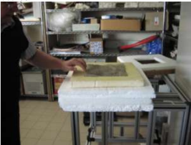
Figure 3: Measuring Sample without line thermal protection
