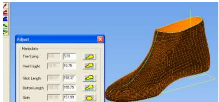
Figure 4: The dimensions of the shoe last with the option to reshape a last
